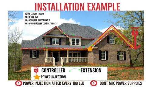
3. Power source in middle lines with 3 separate lines
